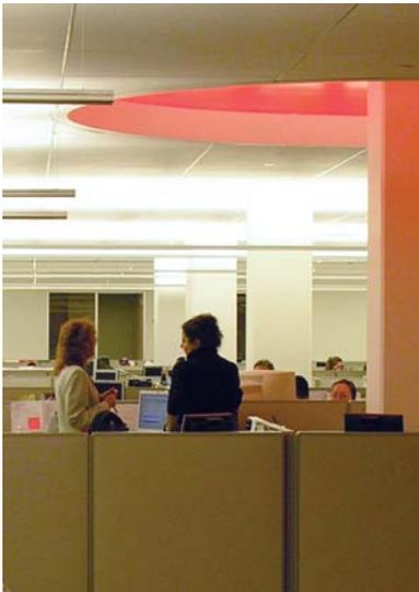
sound-reflecting windows to provide as much natural light into the open plan area as possible. Walls and new domes, fashioned to look like skylights, also reflected sound. The requirement to re-use existing 42" cubicle partitions, while facilitating worker collaboration, would further degrade workplace acoustics.
